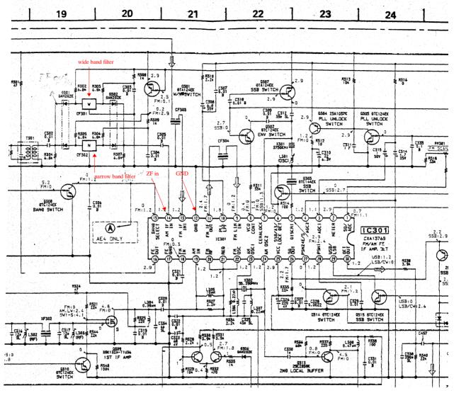
The IF section has two IF filters, a narrow band filter and a wide band filter. One of these filters has to be replaced by a wider filter with appr. 10 kHz bandwidth. The filter 'W' is active if the receiver is in 'wide' mode, the filter 'N' is active if the receiver is in 'narrow' mode.
